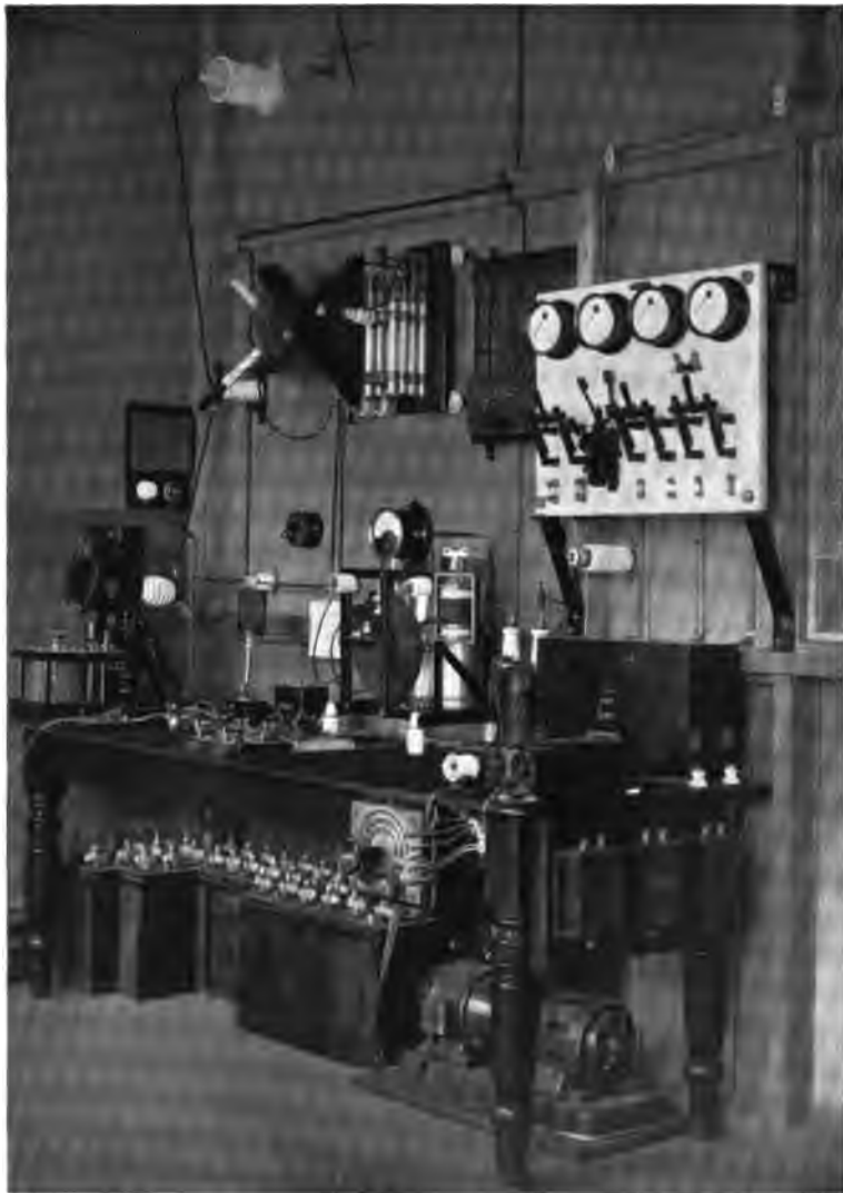
A Quenched-Spark land station, erected by Messrs. Siemens Bros. Ltd., at Cardiff. [ Optispiece. ] [See p. 277.]
